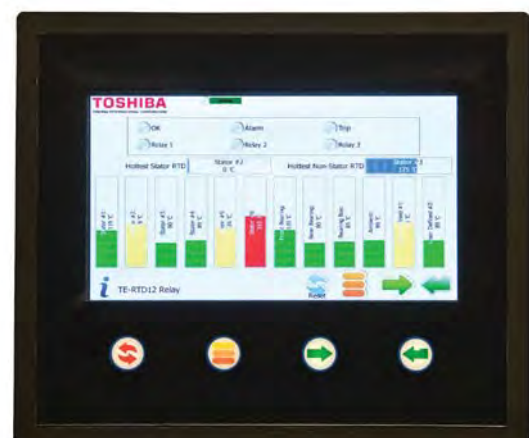
Touchscreen showing TE-RTD Relay with all 12 RTD temperatures.
