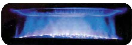
Axial Magnetic Field Interrupter - Arc Dispersion
