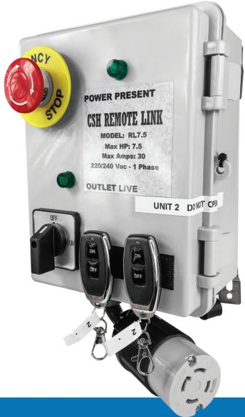
For motor or electrical item requiring starting from distance of up to 320 foot (distance may vary depending on interferences with walls of equipment). The CSH Remote Link is a Non fused manual "ON/OFF" switch as well as a remotely capable switching device for equipment like: Electric motors, Pumps, Lights and other electrical items.
